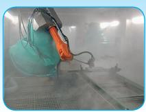
Robotic cleaning of skids at automotive plant. 100 lpm / 1000 bar  $\,$
